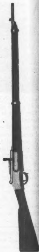
The Comblain Brevete rifle has a large bolt handle above the magazine which pulls up to break the toggle joint. The initial movement of the handle lifts the locking block out of the receiver and the full stroke withdraws the bolt fully, indexing the magazine one compartment
